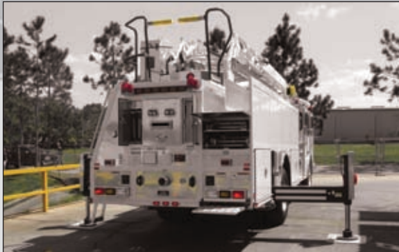
Pin-free jack system deploys in under 40 seconds
